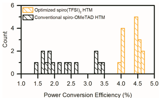
Figure 6. Histogram of ssDSSCs containing either an optimized 12 mol % spiro(TFSI) 2 /tBP HTM or a conventional spiro-OMeTAD/tBP/LiTFSI HTM. All devices were fabricated in a nitrogen atmosphere post-sensitization. Reported efficiencies for conventional devices were obtained in air while those of spiro(TFSI) 2 -based devices were obtained in a nitrogen atmosphere. Fifteen devices per HTM formulation (0.1% bin size).
